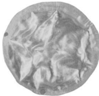
Figure 23.10. Photograph of the Pd membrane creased immediately after ^3\text{H}_2 charging.
