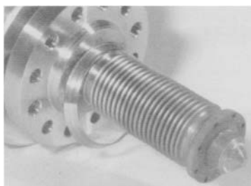
Figure 4.35. Crevice corrosion along valve bellows and flange gap.
