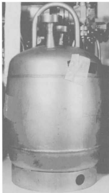
Figure 4.19. Deformation of a storage container by high radiolytic pressure.
