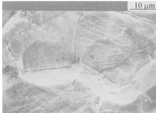
Figure 3.4. Embrittlement accompanied by cracking at the titanium grain boundaries and fine striations resembling cleavage by tritium gas dissolved in tritiated water.
