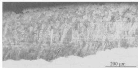
Figure 5.14. Micrograph of a typical coating made using a laser beam.
