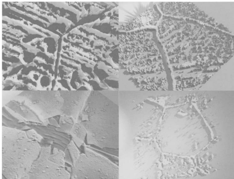
Figure 25.4. 3D surface morphology, (left top): pits and grain boundaries corrosion, (right top and right bottom): grain boundaries corrosion, (left bottom): cracked oxide.
