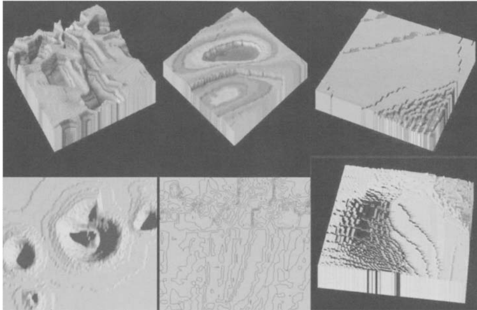
Figure 25.18. Localized corrosion, (left top): three dimensional topographic view showing cracks and pits, (middle top): three dimensional topographic view showing pits, (right top): three dimensional topographic view showing contours of deformed oxide, (left bottom): planar view showing pits, (middle bottom): contours visualization of image in the left top, (right bottom): three dimensional topographic view showing contours of deformed oxide.
