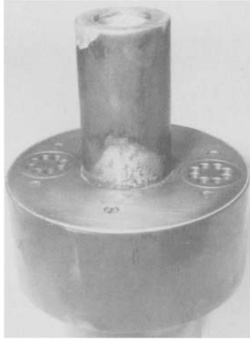
Figure 4.29. Photograph showing salting out phenomena in turbomolecular pump parts.
