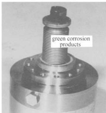
Figure 4.34. Galvanic corrosion between stainless steel flange and copper seal.
