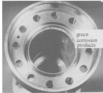
Figure 4.33. Galvanic corrosion between stainless steel flange and copper seal.
