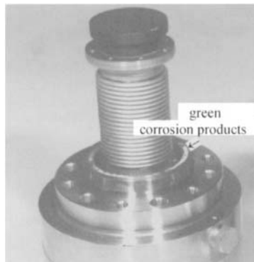
Figure 4.16. Photographs of the corrosion points in tritium installations observed during maintenance or in dismantling. Plate 3: galvanic corrosion for the copper seal and stainless steel valve assembly.
