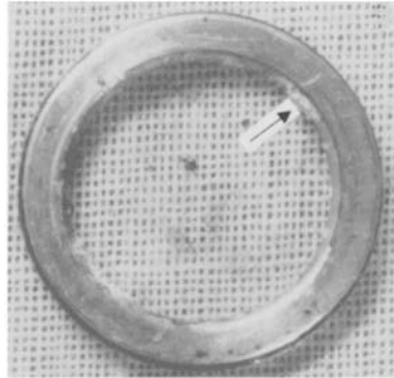
Figure 4.14. Photographs of the corrosion points in tritium installations observed during maintenance or in dismantling. Plate 1: joint elements on which corrosion by recess effect was observed (arrows).
